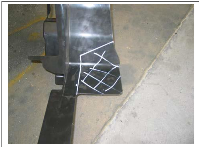
Figure 1: Trim area on passengers side of vehicle. Drivers side is an identical cut.
