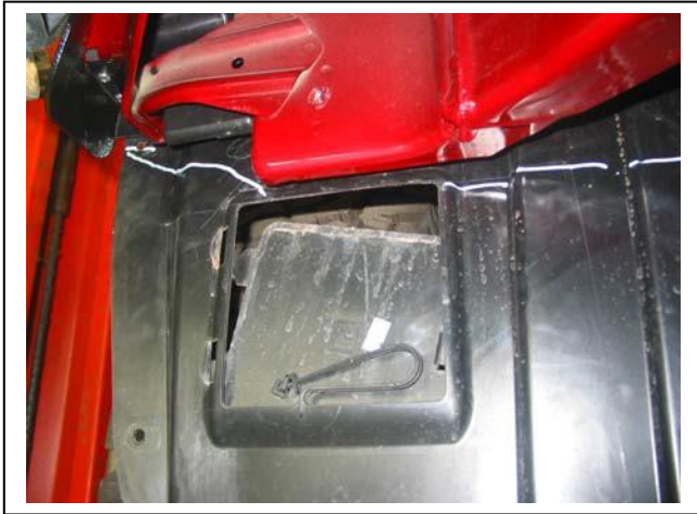
Figure 5: Driver side inner guard trim line.
