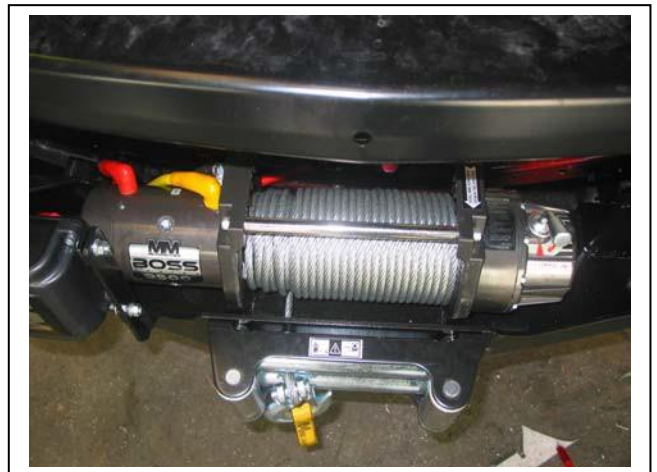
Figure 7: Install winch in winch frame as per manufacturers instructions
