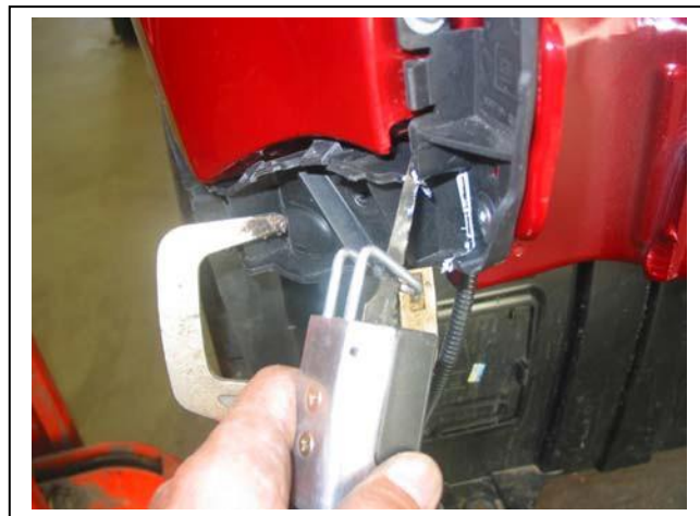
Figure 3: Trim lower bumper keeper to front corner of guard
